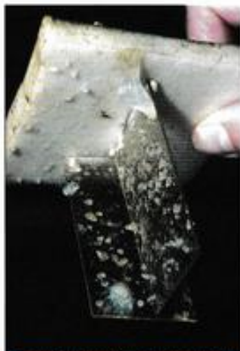
Two glass plates (each 2 x 45 cm) are mounted in styrofoam. Here they are seen after being left for several weeks in the sump of a reef aquarium.
